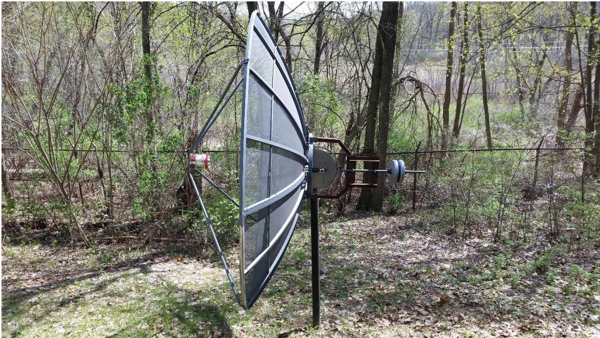
MHAS 3m Dish Antenna, Repurposed from a C-Band Satellite TV Receiving System (1980's Vintage)
