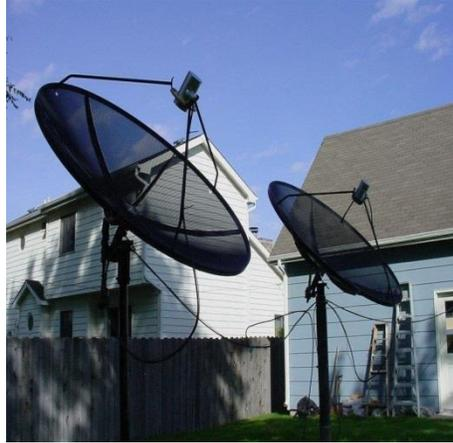
Finally, a surplus Ku band TV satellite dish (Dish Net or Direct TV dish) can be made into an "Itty Bitty Telescope" (IBT) to demonstrate the principles of thermal emission from bodies at room temperature, such as trees, cars, humans, and so on at the operating frequency of around 12 GHz.
